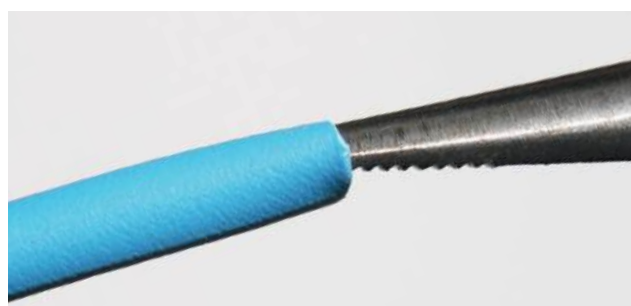
4 Tuck the cut end inside the new tubing
